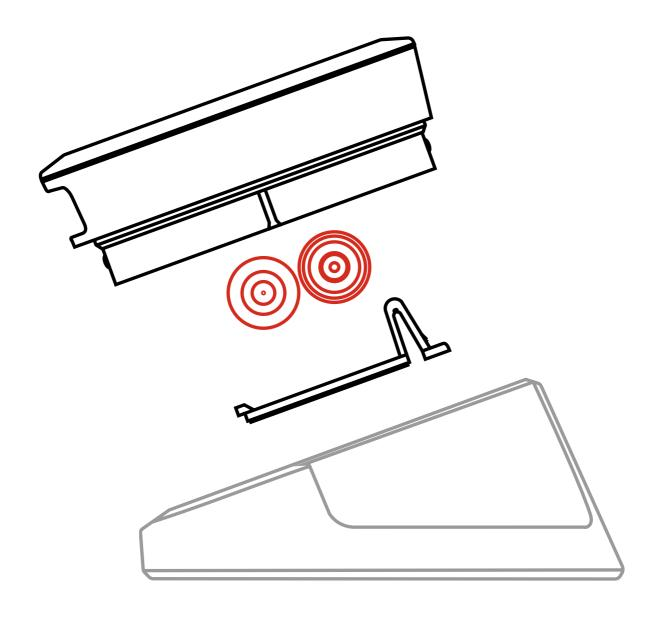
Remove top unit from base, insert batteries
