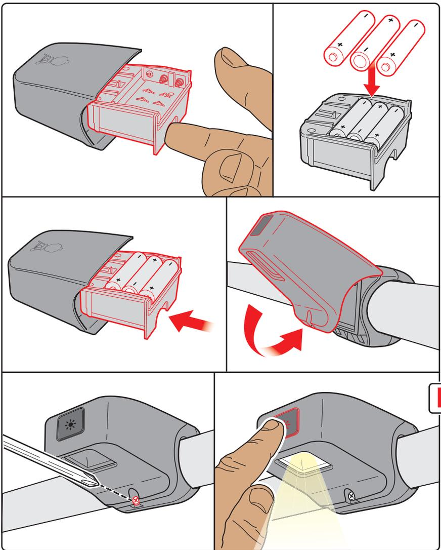
Before use, the grill light should be positioned as shown in illustration **(a)**. Press the AWAKE button to activate the grill light. The light has a 'tilt sensor' that will turn on the light if the grill lid is opened and turn off the light when the grill lid is closed. If the lid is left open or closed for more than 30 minutes, the grill light will deactivate. To turn the light back on, press the AWAKE button **(b)**.
