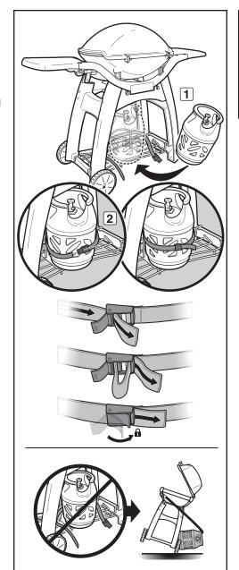
Maximum LPG cylinder capacity when INSTALLED ON CART under the grill is 6 kg.
