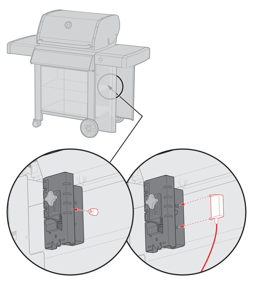
Ensure tank scale has one magnet installed.
