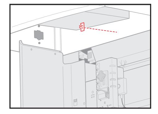
▲ Must secure all wires using the wire retention clip.
