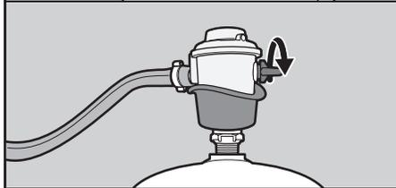
**⚠ DANGER:** Do not use a flame to check for gas leaks. Be sure there are no sparks or open flames in the area while you check for leaks.
