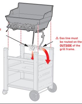
$\triangle$  Route wires to the outside of the corrugated gas line.
