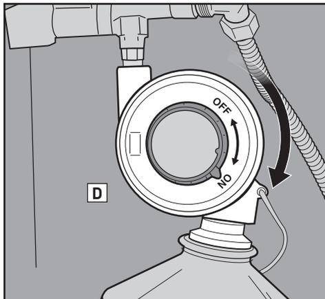
*NOTE: The burner is only meant for igniting charcoal, not for cooking. Turn burner control knob off promptly after charcoal is lit to preserve the fuel in your disposable cartridge. Turn gas supply off at the source.*
