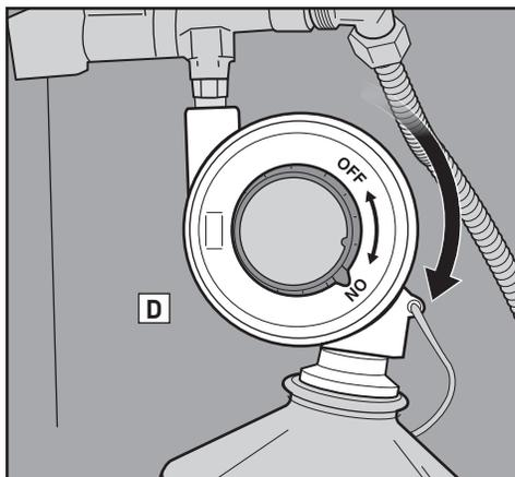
**⚠ WARNING: If burner fails to ignite within five seconds, stop, turn the burner control knob to off, and wait five minutes to allow the gas to clear before you try again or light with a match.**
