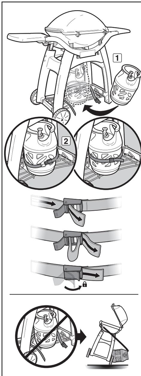
**Maximum LPG cylinder capacity when INSTALLED ON CART under the grill is 6 kg.**
