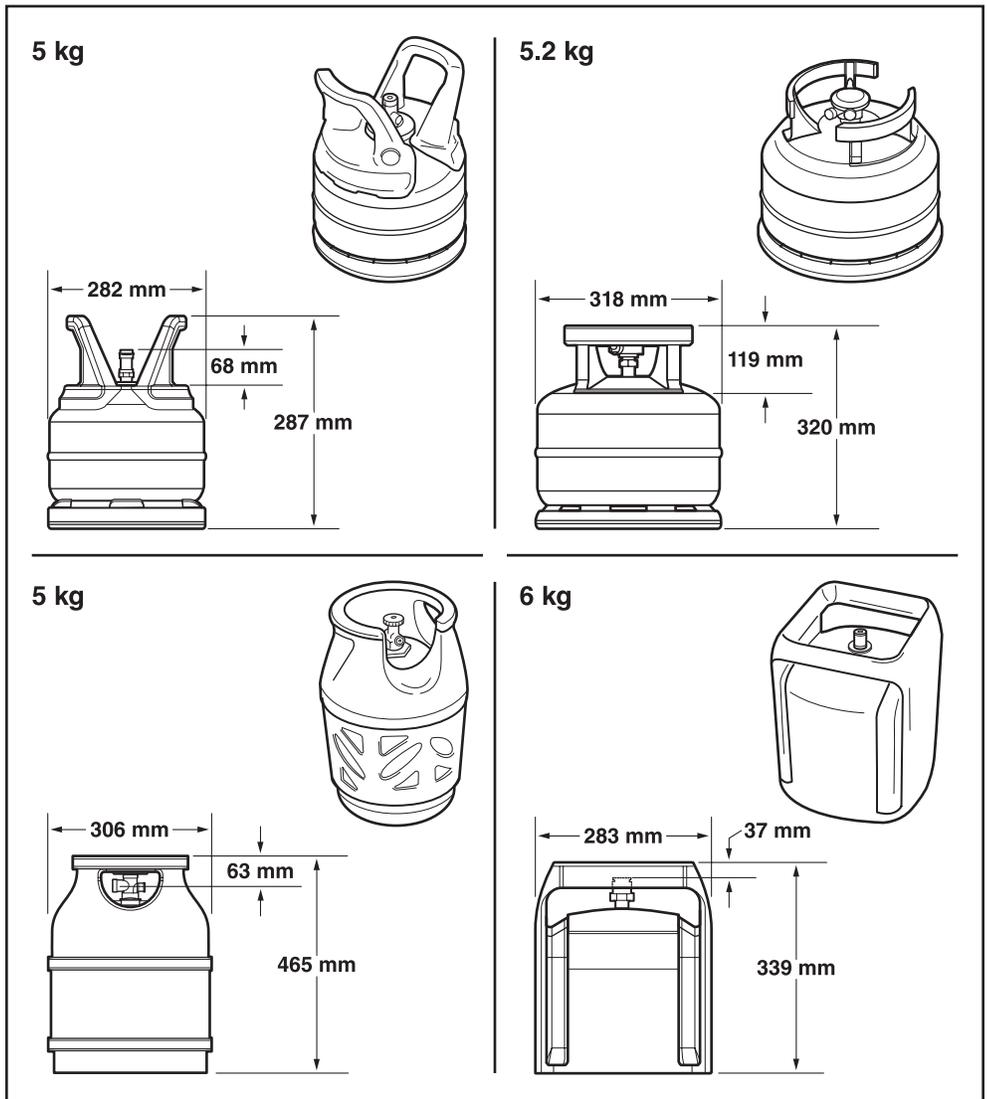
**Maximum LPG cylinder capacity INSIDE cabinet is 6 kg.
