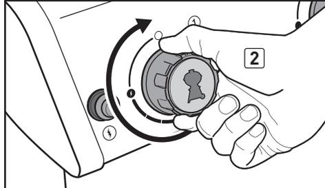
C) Turn on the cylinder valve using one of the appropriate options based on your cylinder and regulator type. Refer to "A)" in "CHECKING FOR GAS LEAKS."
